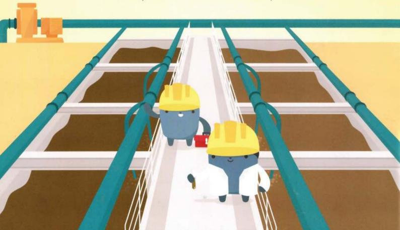
Grease and oils float to the top and are removed while sludge settles on the bottom.
